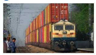
Indian Railways has created a world record by commissioning the first high rise **Over Head Equipment (OHE)** and successfully running **double stack containers** in electrified territory. Rail freight is being used increasingly to compensate for decreased road transport.
